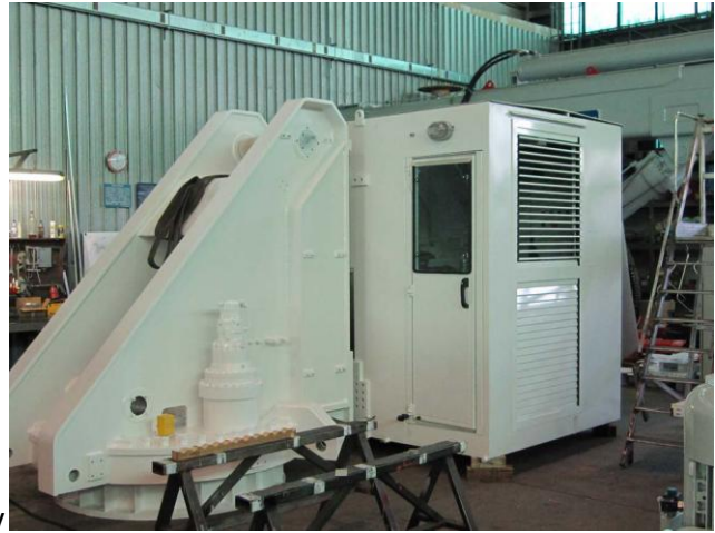
Crane Cabin and Turret Assembly
